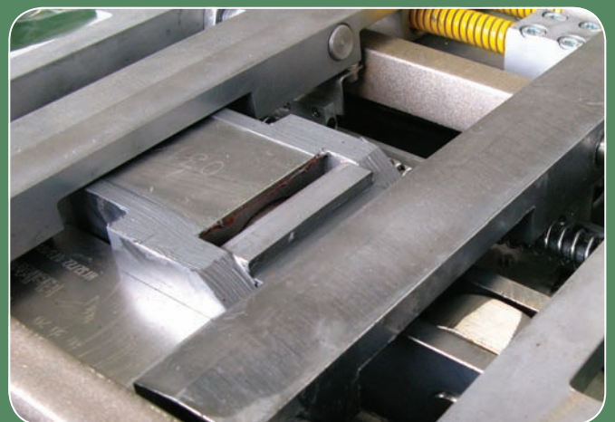
Trailing mechanism is integrated within the lock body
