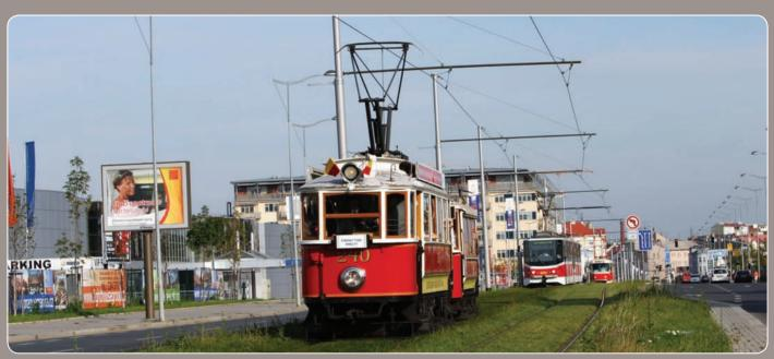
The type of overhead contact line gets chosen also with regards to the aesthetical point of view. For city centres we prefer a simple system suspended by means of DELTA suspension or a simple wire system. This option offers an aesthetical... ...and silent solution maintaining the elasticity, high operation speed, and low number of poles.
