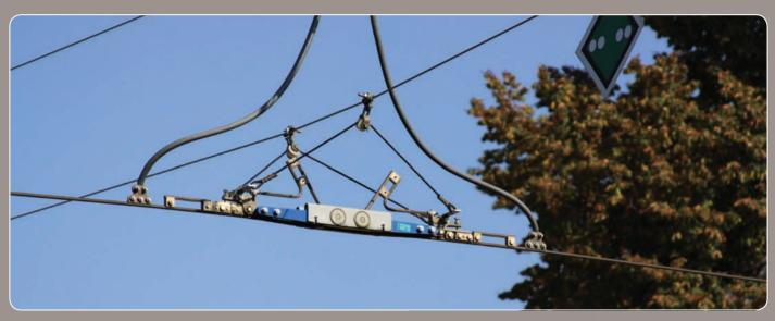
A special construction of our section insulators allows a silent and fast passage of the pantograph. Our section insulators are designed in such a way to safely interrupt both common equalizing currents and contingent short-circuit currents.
